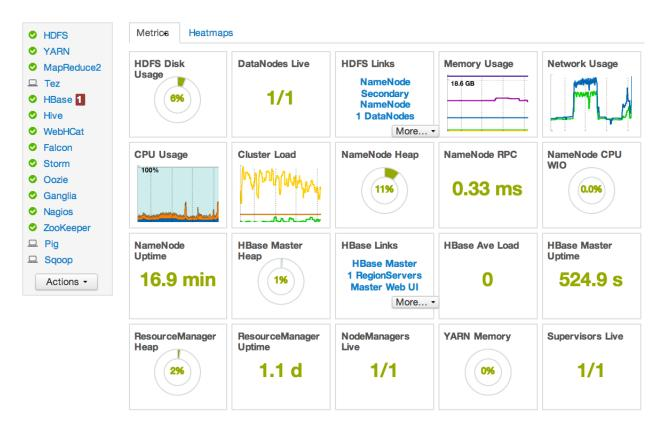
Status information appears as simple pie and bar charts, more complex charts showing usage and load, sets of links to additional data sources, and values for operating parameters such as uptime and average RPC queue wait times. Most widgets displays a single fact by default. For example, HDFS Disk Usage displays a load chart and a percentage figure. The Ambari Dashboard includes metrics for the following services:
