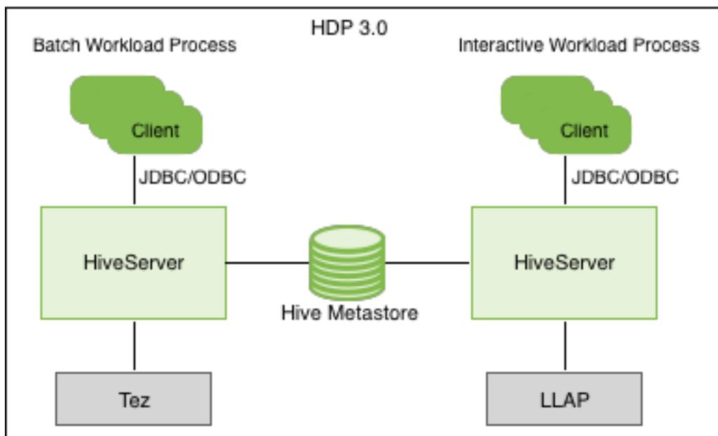
You can connect to Hive using a JDBC command-line tool, such as Beeline, or using a JDBC/ODBC driver with a BI tool, such as Tableau. Download the JDBC driver `hive-jdbc` from the <https://www.cloudera.com/downloads/hdp.html>. Clients communicate with an instance of the same HiveServer version. You configure the settings file for each instance to perform either batch or interactive processing.
