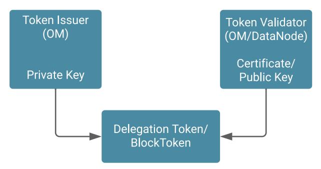
In secure mode, SCM bootstraps itself as a certifying authority (CA) and creates a self-signed CA certificate. OM and DataNode must register with SCM CA through a Certificate Signing Request (CSR). SCM validates the identity of OM and DataNode through Kerberos and signs the component's certificate. The signed certificates are then used
