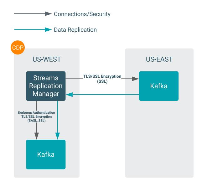
There are two clusters, US-West and US-East. US-West is a Cloudera cluster that has both Kafka and Streams Replication Manager deployed on it. The Kafka service on this cluster is both Kerberos and TLS/SSL enabled. That is, clients connecting to this cluster (including Streams Replication Manager) use the SASL\_SSL protocol.
