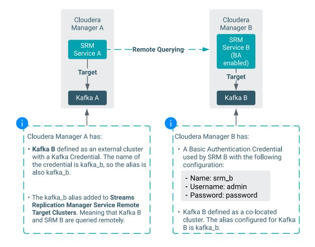
In this specific example, a single Streams Replication Manager Service Credential must be created in Cloudera Manager A. This credential represents Streams Replication Manager Service B and will be used by Streams Replication Manager Service A to access Streams Replication Manager Service B. The credential would be configured as follows:
