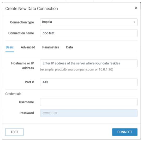
In this example, the Impala connection is made through Knox. Knox always uses TLS encryption and port 443 is the default HTTPS port.
