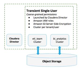
Twice a week, a member of the **etl\_team** uses Altus Director to launch EC2 instances, spins up the cluster, runs the workload, and then shuts down the cluster when the workload completes. As the job runs on the cluster, results are written back to Amazon S3 to the etl-results bucket.
